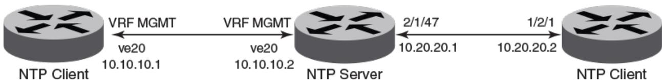
In this scenario, the NTP server has one client using Management VRF and one client using an Ethernet port.
