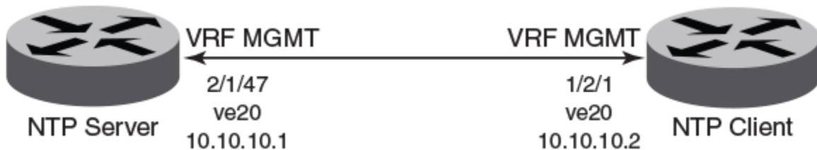
In this scenario, NTP over Management VRF is implemented on both an NTP server and an NTP client device using Virtual Ethernet (VE) interfaces.
